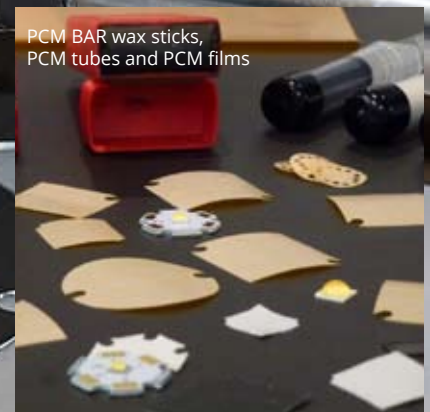
Specific LED cuts of electrically insulating and non-insulating PCM films at our production facilities
